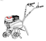
3.1.3 Remove the circlip B on the front wheel support rod, adjust the front wheel support rod upward to another position, and then install the circlip B.
